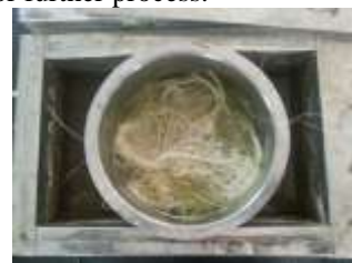
Figure 2.1 : Softening of Sisal Fibre
